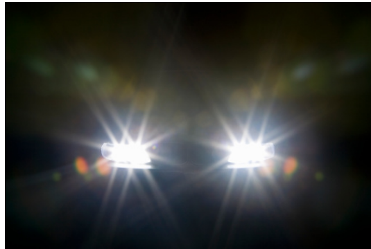
Figure 4: Example of headlights being a glare source, resulting in starbursts and causing discomfort and potentially disability glare
